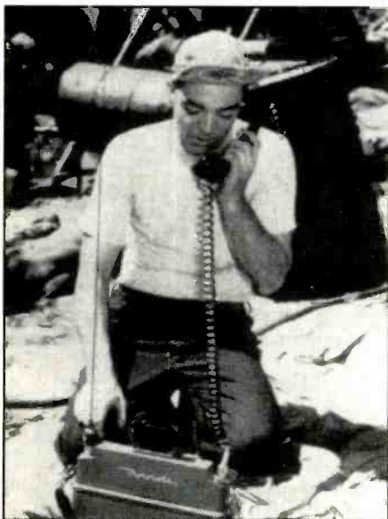
The first commercial two-way FM portable was developed by Motorola in 1947. It used miniature tubes.
