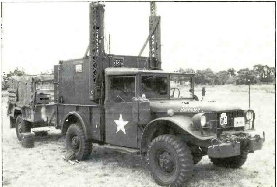
The twin towers are always retracted when the vehicle is in motion.
