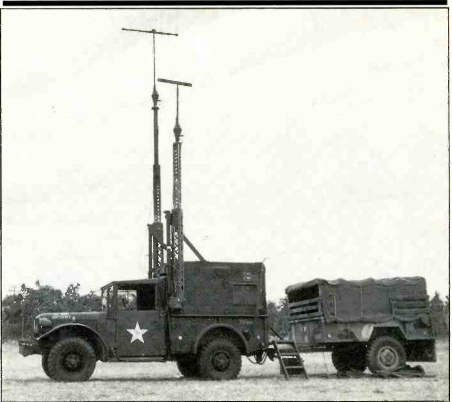
The utility trailer also contains the generator.
