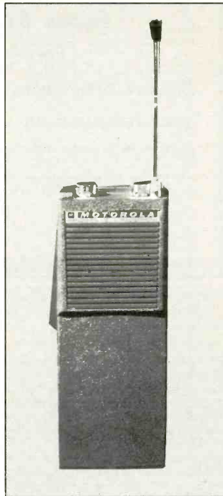
The Motorola HT200, introduced in 1962, was the first fully transistorized FM two-way portable.
